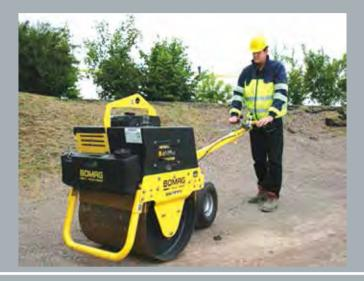
**Specifications:** Brand Name: BOMAG Model No.: BW 71 E-2 -Walk-Behind Single Drum Vibratory Roller Operating Weight: 488 kg Working Width: 410 mm Quantity: 3
