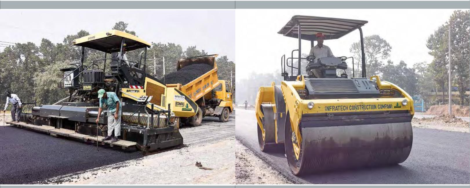
Specifications: Brand Name: BOMAG Model No.: BF 800C S600 Max Width: 10 m Max Power: 180 hp Operating Weight: 21300 kg Quantity: 2
