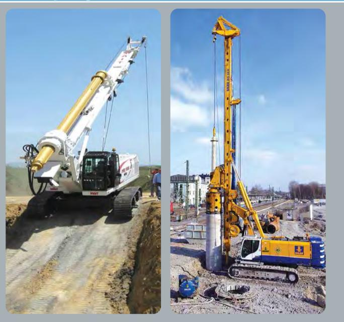
**Specifications:** Brand Name: MAIT Model No.: HR-30/3 Max Depth: 22 m Max Diameter: 900 mm Max Torque: 35 KNm Qty: 2
